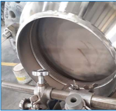
FCAW Overlay on Flange ID
