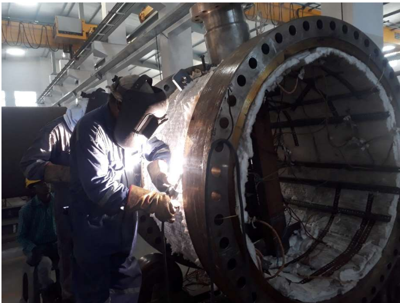
Heavy thickness Job (5Cr, 1Mo) being welded with electrical Pre-heating, Local Furnace for Refractory Drying
