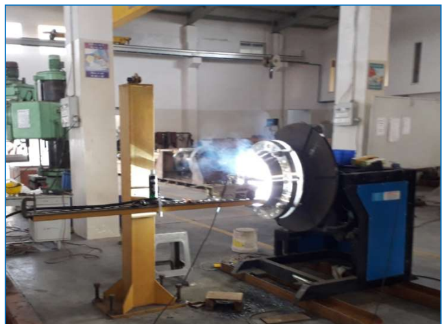
FCAW Overlay Welding Work Station
