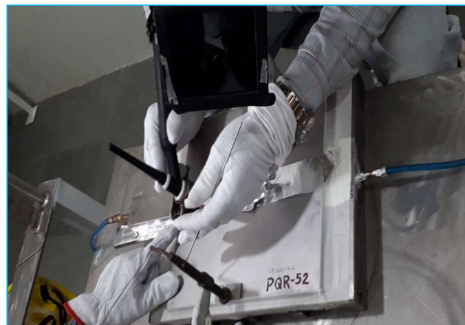
Titanium Welding Carried out using Trailing
