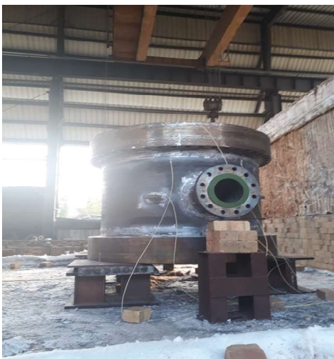
Channel Head before firing, On Furnace bed
