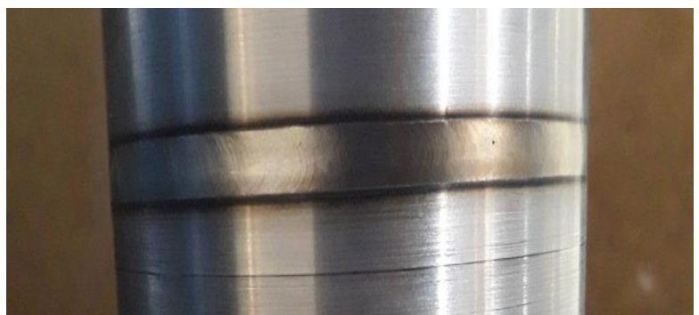
Weld using Autogenous TIG Process
