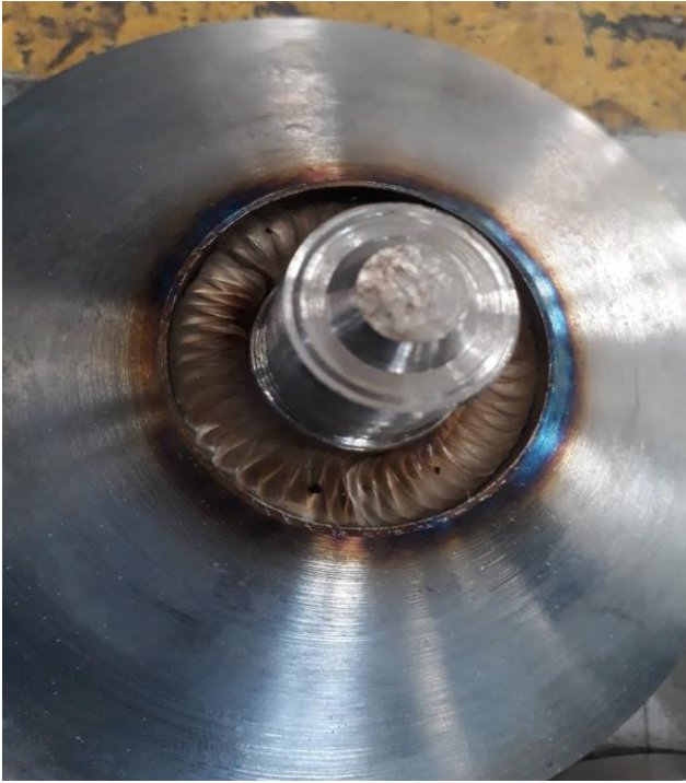
Stellite Weld overlay on Inconel
